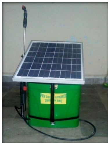
Fig. 2: Solar cum hand operated hybrid knapsack sprayer
